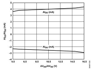
Figure 20. Supply Current vs. Supply Voltage (Dual Supply)
