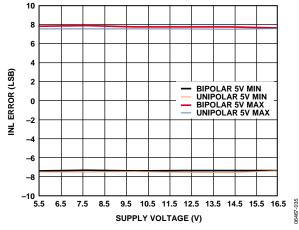
Figure 15. AD5752 Integral Nonlinearity Error vs. Supply Voltage
