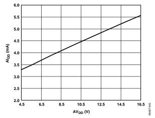
Figure 21. Supply Current vs. Supply Voltage (Single Supply)
