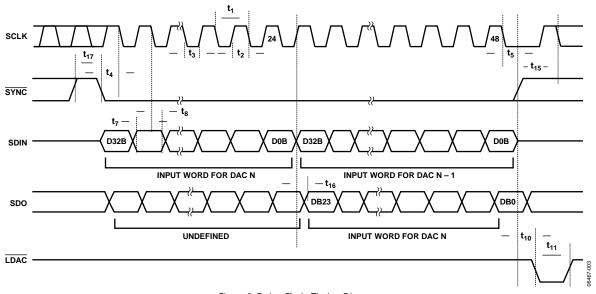
Figure 3. Daisy-Chain Timing Diagram
