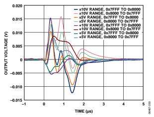
Figure 31. Digital-to-Analog Glitch Energy
