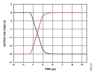
Figure 28. Full-Scale Settling Time, ±5 V Range
