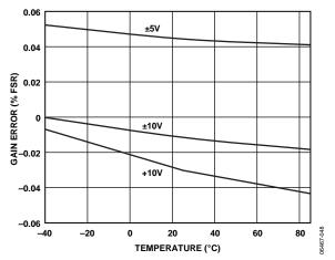
Figure 24. Gain Error vs. Temperature
