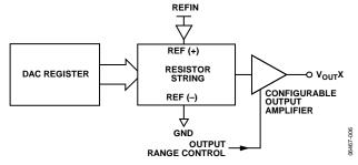
Figure 38. DAC Architecture Block Diagram
