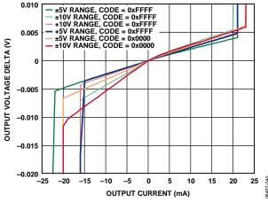
Figure 26. Output Source and Sink Capability
