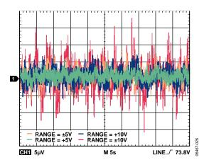
Figure 32. Peak-to-Peak Noise, 0.1 Hz to 10 Hz Bandwidth
