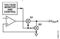
Figure 42. Analog Output Control Circuitry
