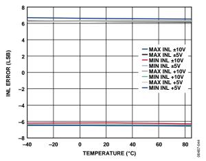
Figure 12. AD5752 Integral Nonlinearity Error vs. Temperature
