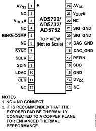
Figure 5. Pin Configuration
