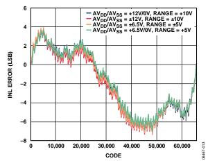
Figure 6. AD5752 Integral Nonlinearity Error vs. Code
