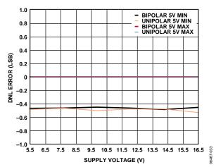
Figure 17. AD5752 Differential Nonlinearity Error vs. Supply Voltage
