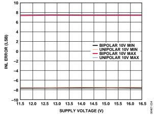
Figure 14. AD5752 Integral Nonlinearity Error vs. Supply Voltage
