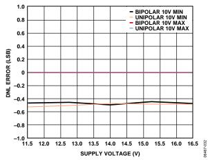
Figure 16. AD5752 Differential Nonlinearity Error vs. Supply Voltage
