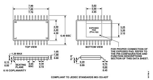
Figure 45. 24-Lead Thin Shrink Small Outline Package, Exposed Pad [TSSOP\_EP] (RE-24) Dimensions shown in millimeters
