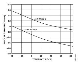
Figure 23. Bipolar Zero Error vs. Temperature
