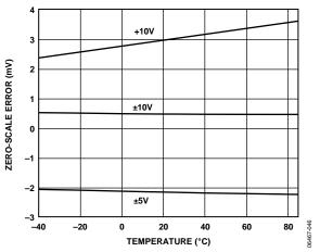
Figure 22. Zero-Scale Error vs. Temperature
