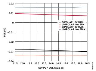
Figure 18. AD5752 Total Unadjusted Error vs. Supply Voltage
