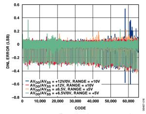
Figure 9. AD5752 Differential Nonlinearity Error vs. Code
