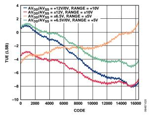
Figure 36. AD5732 Total Unadjusted Error vs. Code
