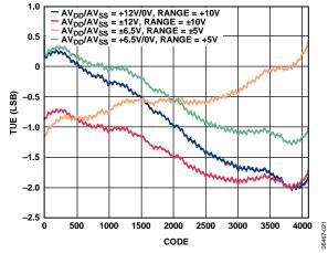
Figure 37. AD5722 Total Unadjusted Error vs. Code
