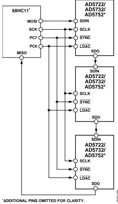
Figure 40. Daisy Chaining the AD5722/AD5732/AD5752
