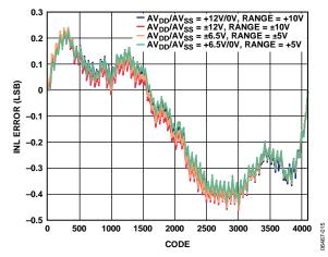
Figure 8. AD5722 Integral Nonlinearity Error vs. Code
