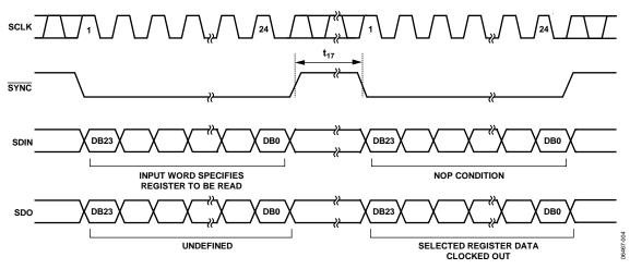
Figure 4. Readback Timing Diagram
