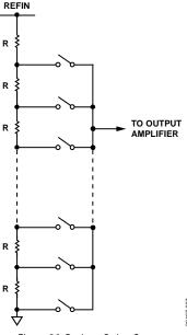
Figure 39. Resistor String Structure
