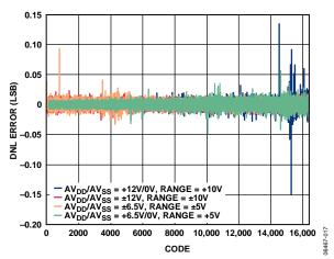
Figure 10. AD5732 Differential Nonlinearity Error vs. Code
