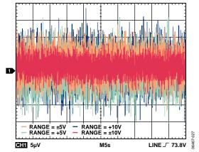
Figure 33. Peak-to-Peak Noise, 100 kHz Bandwidth
