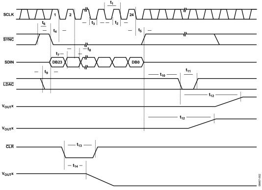
Figure 2. Serial Interface Timing Diagram
