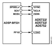
Figure 44. AD5722/AD5732/AD5752 to Blackfin Interface
