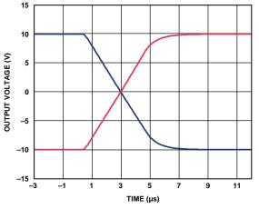
Figure 27. Full-Scale Settling Time, ±10 V Range
