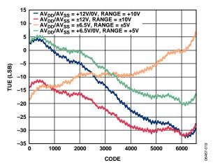
Figure 35. AD5752 Total Unadjusted Error vs. Code
