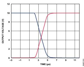
Figure 29. Full-Scale Settling Time, +10 V Range
